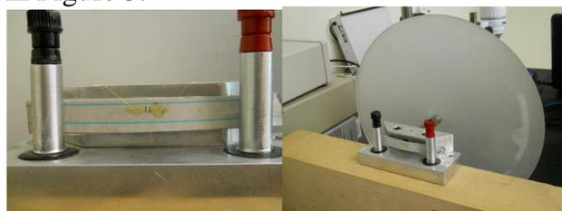
Figure 3: the gold wire attached to the metal strip and then put in the bending apparatus.
