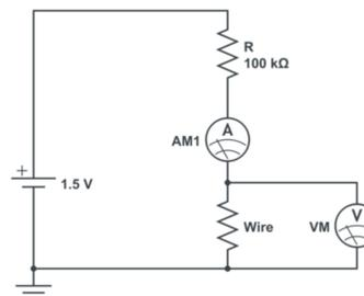
Figure 4: Circuit diagram used for both the MCBJ and etching techniques. The wire was notched so when the disk was bent, the wire would splinter and create a nanocontact.
