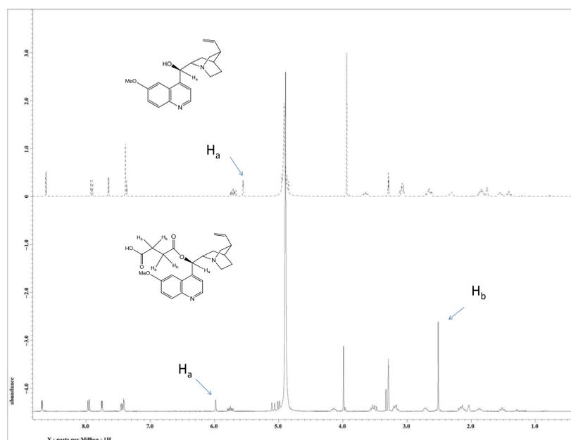
Figure 2.  $^1\text{H-NMR}$  overlay spectra of quinine and quinine hemisuccinate in  $\text{CD}_3\text{OD}$ .
