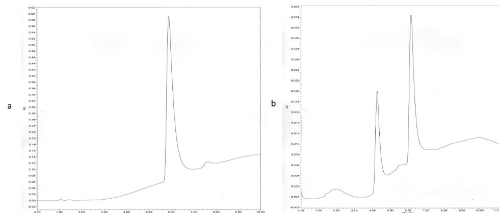
Figure 3 a) HPLC spectrum of unmodified quinine. b) HPLC spectrum of quinine hemisuccinate. Note difference in y-axis scaling compared to 3a.
