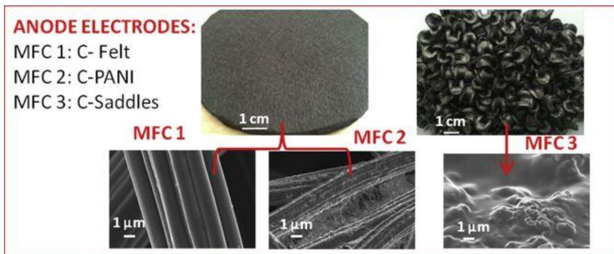
**Figure 3.** A macroscopic and microscopic view of carbon felt, carbon felt with polyaniline, and carbon-coated Berl saddles. Note the difference in appearance and texture.<sup>7</sup>
