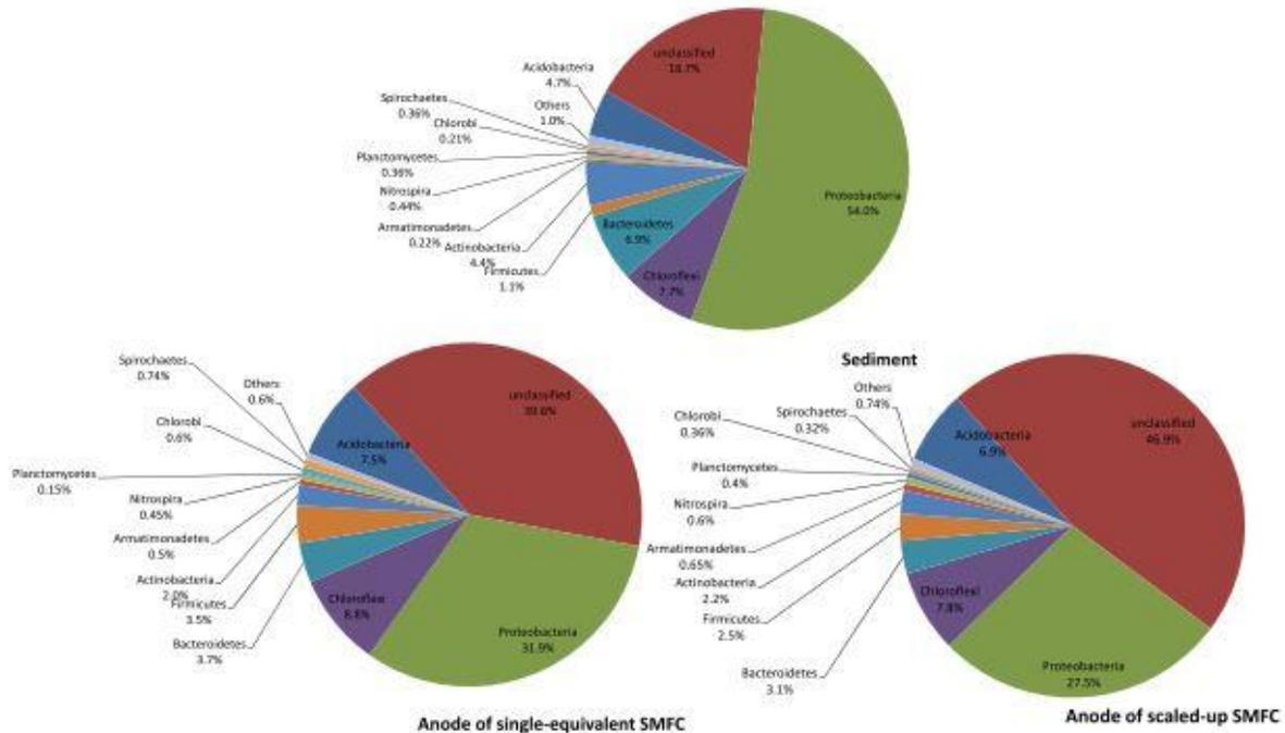
**Figure 4.** “Microbial community structure at the phyla level on anodes of the single-equivalent SMFC and the scaled-up SMFCs compared with the original sediment community.”<sup>2</sup>
