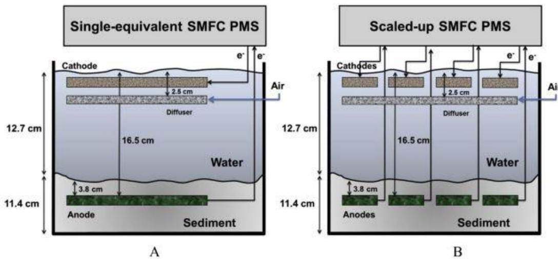
**Figure 11.** Schematic of (A) a single-equivalent SMFC and (B) a scaled-up SMFC.<sup>2</sup>
