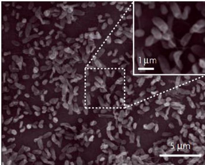
**Figure 8.** “Scanning electron micrograph of *Rhodospseudomonas palustris* on a carbon paper anode.”<sup>11</sup>
