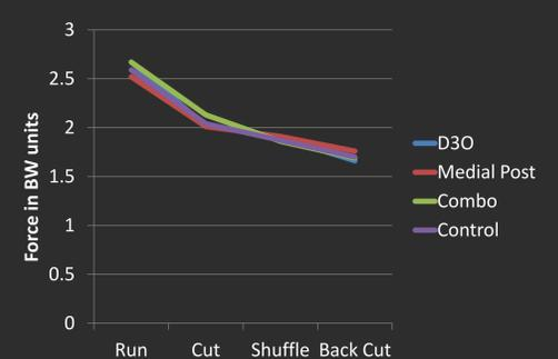
Figure 5: Men Maximal Vertical Force by Shoe
