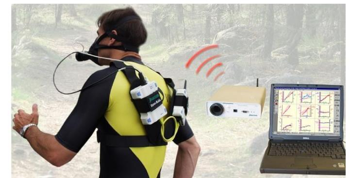
Figure 3. The Oxycon Mobile, a portable metabolic analyzer.
