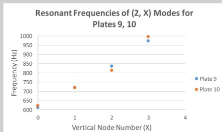
**Figure 6** A comparison of resonant frequencies of (2, X) modes between a stressed plate (Plate 10) and an unstressed plate (Plate 9) of the same shape.
