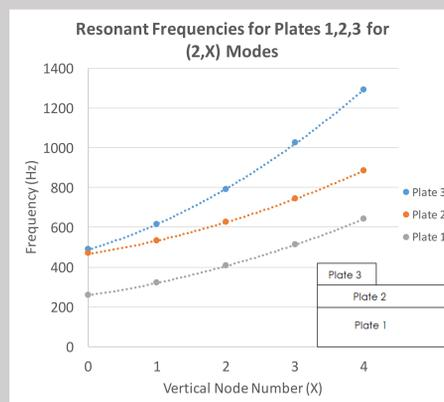
**Figure 3** A plot of resonant frequencies for (2, X) Modes. Plate 3 is the smallest, Plate 1 is the biggest, and Plate 2 is in between.
