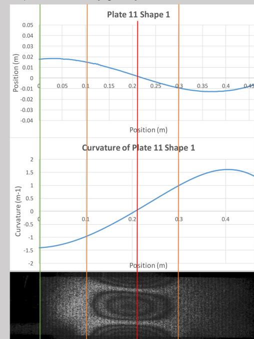
**Figure 5** The top is a digitized tracing of the shape Plate 11's curve. The middle is a plot of the curvature of the shape. The bottom is an ESPI image of the plate resonating at the (2,0) mode. The green lines denote the edges of the plate. The orange lines denote the edges of the pattern of vibration. The red line denotes where the curvature is zero.
