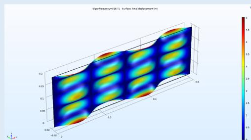
**Figure 2** A COMSOL image representing the same (4,3) Mode as Figure 1. The blue lines in COMSOL images represent the nodal lines.
