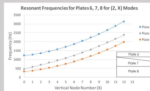
**Figure 4** A plot of resonant frequencies of (2, X) Modes for a tapered plate and two rectangular plates.
