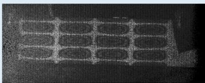
**Figure 1** ESPI Image of a plate vibrating at its (4,3) Mode. Mode numbers are denoted by the horizontal (4) and vertical (3) nodal lines, excluding the ends. White lines in ESPI images represent the nodal lines.
